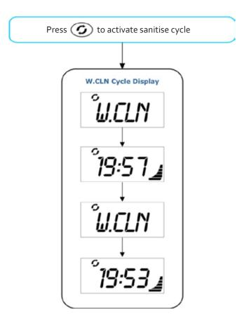
Whilst the cycle is running the display alternates between the W.CLN (water clean) title screen and the minutes remaining in the cycle (refer above).
