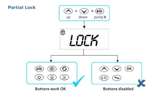
The keypad buttons can be locked to prevent accidental key presses or to limit access to certain controller functions. This feature is particularly helpful when spa covers are used or where children are present.
