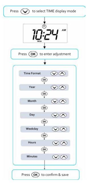
Be sure to set the date and time before operating the spa. Vital functions such as filtration, sanitisation cycles and power saving settings depend on the time and date being set correctly.
