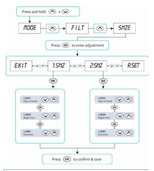
Accessed via the Setup Menu, Sleep timers are a very handy feature that enables the user to stop all spa activity during certain times of day or night. While the controller is sleeping NO automatic heating or filtration maintenance will occur, however the spa can still be operated by manual use without the need to adjust sleep time settings.
